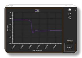
Real-time flare efficiency functionality provides continuous monitoring of the efficiency level for each flare in the field of view of SENSIA's Agni. If an irregular event is detected as defined by customizable settings in RedLook, an alarm will be generated automatically.
