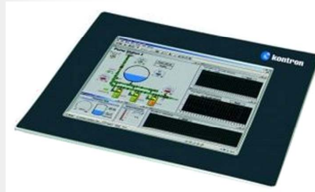
Display for the front door of the control enclosure
