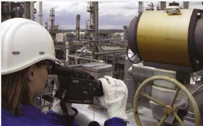
Examining potential leak paths
